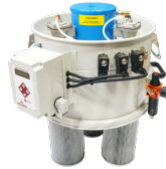
SP Reverse air jet filter cleaning system Antistatic M class filter (EN 60335-2-69), 3 Polyester filter cartridges, 9 m² filter surface
