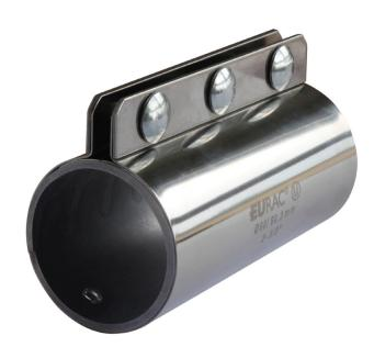
PICO-LM coupling is used for connection of details with straight edges. Length: 150 mm.
